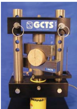
Indirect tension Brazilian test jig.
